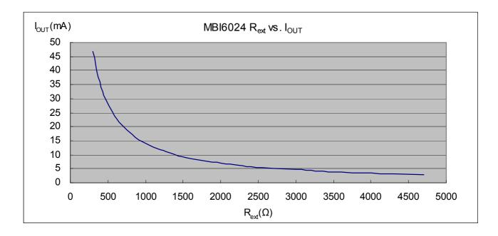
The output current of each channel ( $I_{OUT}$ ) is set by an external resistor,  $R_{ext}$ . When output channels are turned on,  $V_{REXT}$  is around 0.61V. The relationship between  $I_{OUT}$  and  $R_{ext}$  is shown in the following figure.
