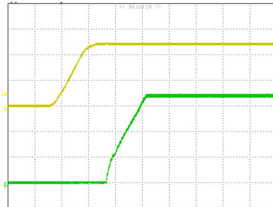
**Figure 13:** Turn on delay time at 12Vin, 1.8V/30A out.
