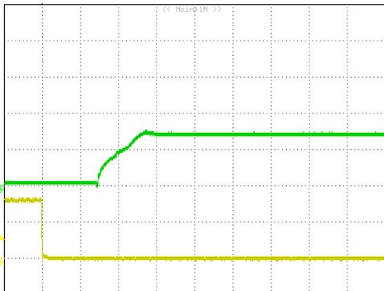
**Figure 16:** Turn on delay time at remote on 12Vin, 0.8V/30A out. (Green: VOUT, 0.5V/div, Yellow: ON/OFF, 2V/div, 1mS/div)
