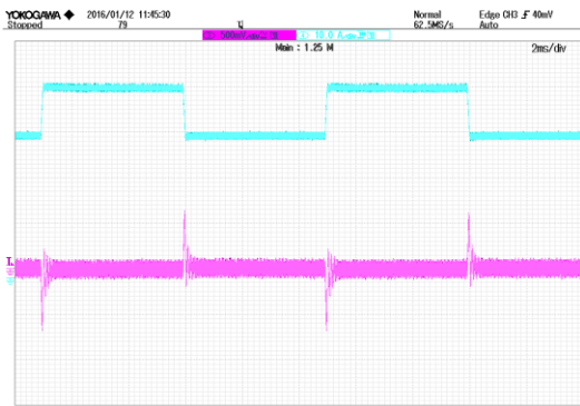
Figure 7: Output voltage response to step-change in load current (75%-50%-75% of full load; di/dt = 0.1A/\mu s ). Top Trace: V_{out} ; 500mV/div; Time: 2ms/div Bottom Trace: I_{out} ; 10A/div; Time: 2ms/div
