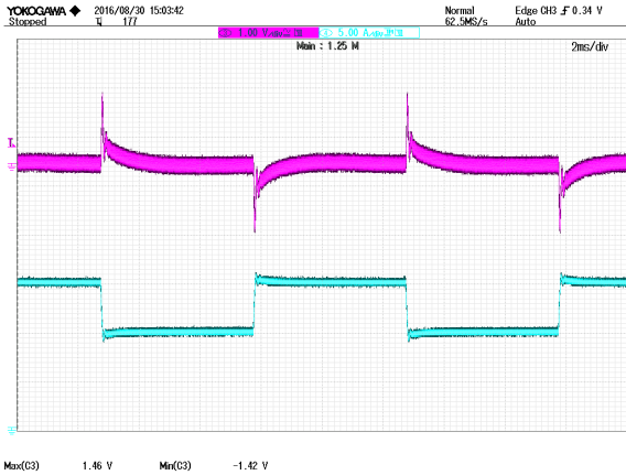
Figure 7: Output voltage response to step-change in load current (50%-75%-50% of full load; di/dt = 0.1A/\mu s ). Top Trace: V_{out} , AC 100mV/div; Time: 2ms/div Bottom Trace: I_{out} , 5A/div; Time: 2ms/div
