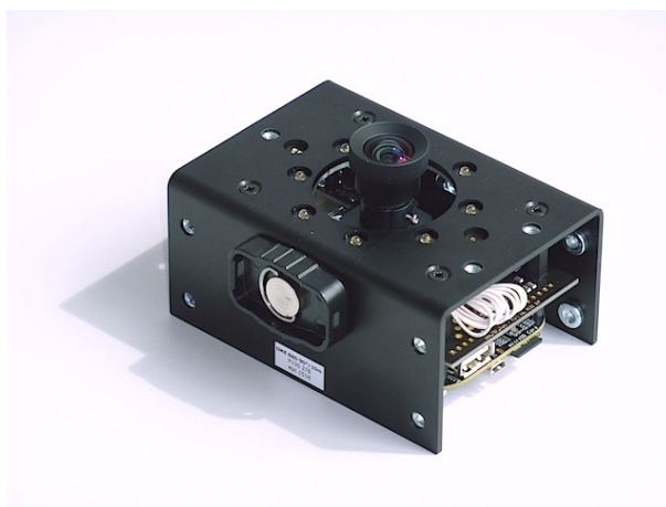
Figure 6: DME 635 with quick release fastener of the tripod
