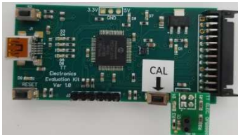
Main and daughter board connection (top view)
