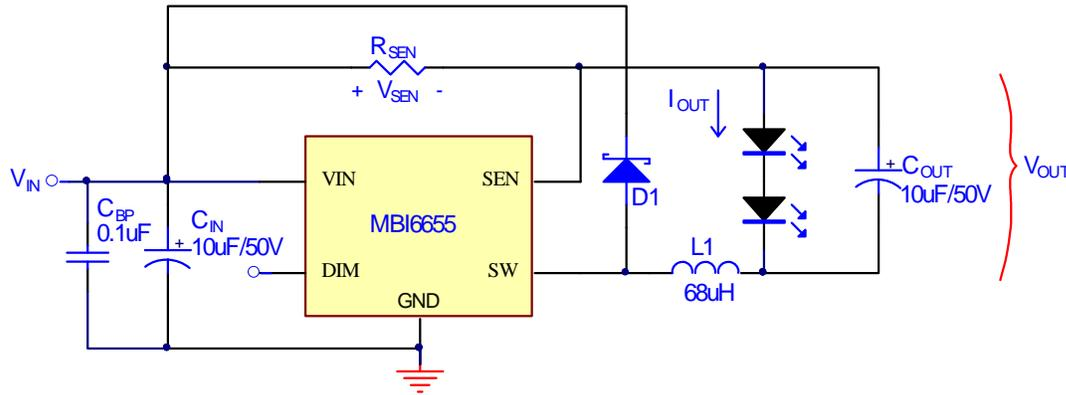
Figure 4 The application circuit of design example
