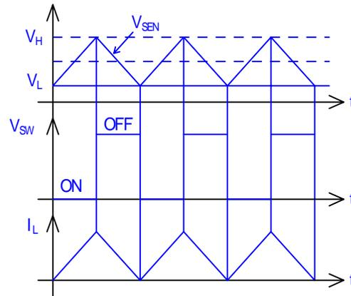
Figure 2. Waveform of hysteretic PFM control scheme
