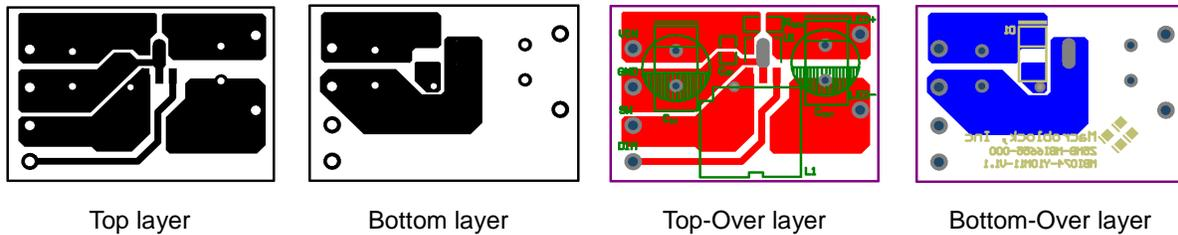
Figure 6. The layout diagram of MBI6655GSB
